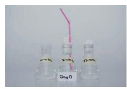
Treatment 1 (T1):CO2 limited - flask covered tightlyTreatment 2 (T2):CO2 fertilised - flask covered with a<br/>cotton wad made airtight by wrapping it<br/>in transparent film with a straw inserted<br/>in the middle for CO2 introduction by<br/>blowingTreatment 3 (T3):control (no CO2 fertilisation) - flask<br/>covered with a cotton wad
