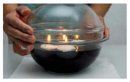
2. Light eight candles and place four in the bowl with frozen distilled water and four in another bowl. Put the four unlit candles in the third bowl. This will serve as your control. Cover the bowls with the remaining empty bowls. Take note of the colour of the water at the start of the experiment.
