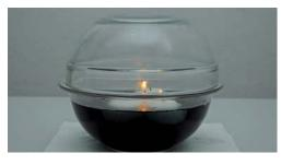
Figure 3 and 4: The bowl with the burning candles is covered with a second bowl. After several minutes, the candles burn out.
